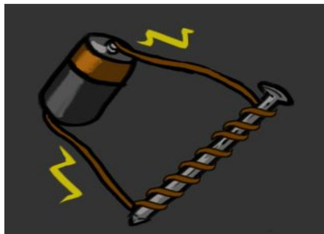
**Step 4:** Now the ELECTROMAGNET is ready. Put the point of the nail near a few paper clips/ other magnetic material and it should pick them up.
