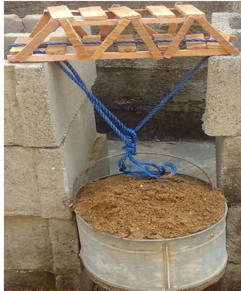
Place load underneath
