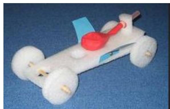
There are many different ways to build a balloon car. Turn this into an engineering design project and try building your car with different materials. For example: *What happens if you use a plastic bottle instead of a carton for the body? What happens if you use different diameter straws or bigger wheels? What about different materials for the wheels and axles?*
