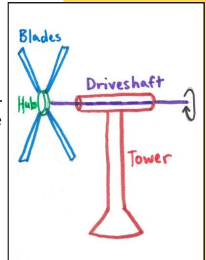
Now, what good is this? What can we do with a spinning driveshaft? In the next activity, students will be building their own simple wind turbines. Our goal will be to get some mechanical work out of our wind turbines: We'll attach a spool, string, and cup to the end of the driveshaft to see if we can lift weights (a few washers.)
