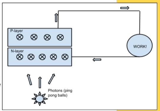
negative charge). The 'p-layer' has some boron added to it, which gives it a tendency to attract electrons (p for positive).
